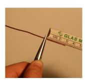
When finished, the wire shold look like this. The mid-to-mid measure should be 31mm, the inside-to-inside measure 29mm. These measures have to be very exact.
