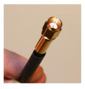
Fasten the connector bushing with the crimping tool.
