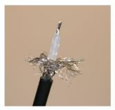
Solder the connector bushing to the inner conductor.
