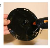
Place the copper wire in the dent you made earlier. The distance between the copper wire and the disc has to be exactly 16mm.
