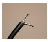
Solder the inner and outer conductor to the antenna as shown.
