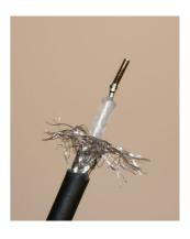
Place the SMA connector on the cable an fold the outer conductor back up.
