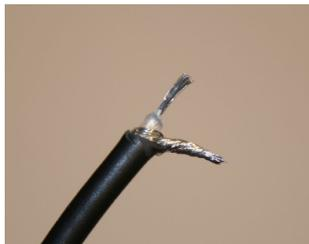
Solder the inner and outer conductor to the antenna as shown.
