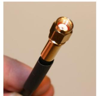
Fasten the connector bushing with the crimping tool.
