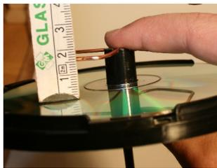
When all is right, secure the antenna by applying melt glue.
