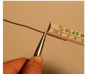
When finished, the wire should look like this. The mid-to-mid measure should be 31mm, the inside-to-inside measure 29mm. These measures have to be very exact.
