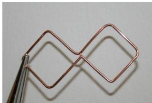
Solder the open ends of the wire together.
