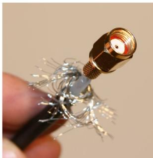
Push the connector bushing over the outer conductor and SMA connector.
