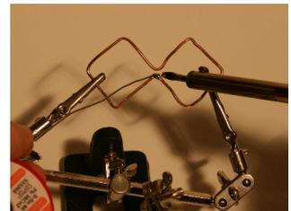
Strip <1cm from one side of the RG58 cable and twist it like shown.
