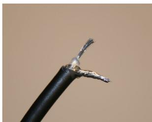
Solder the inner and outer conductor to the antenna as shown.
