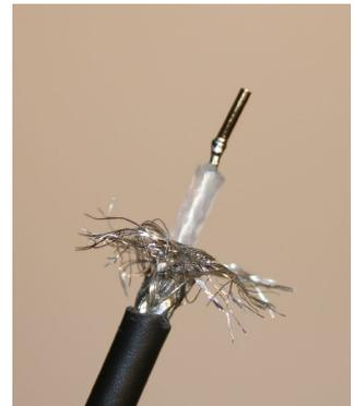
Place the SMA connector on the cable and fold the outer conductor back up.
