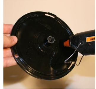
Place the copper wire in the dent you made earlier. The distance between the copper wire and the disc has to be exactly 16mm.
