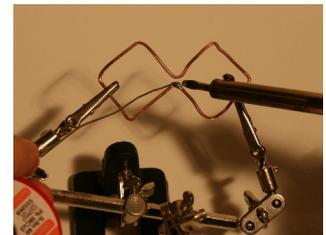
Strip <1cm from one side of the RG58 cable and twist it like shown.
